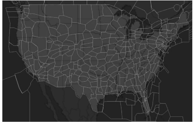
Fig. 1 Current ARTCCs (left), and ATC sectors in continental U.S. airspace (right) (pictures courtesy of Federal Aviation Administration).
